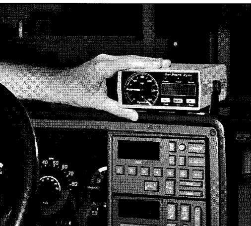
The display unit was positioned directly in the driver's line of view for easy reading.
